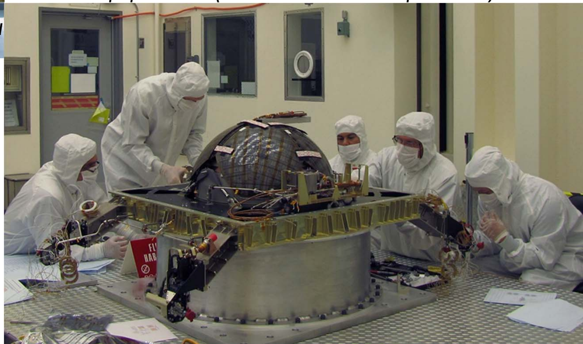
SMAP HR-18 Reaction Wheels have successfully completed random vibration testing (photos courtesy Honeywell)
