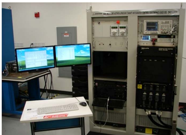
"Hardware in the Loop" aka "HITL" enables closed-loop simulation of spinning Observatory dynamics
