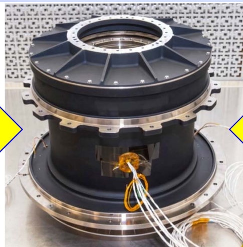
Flight BAPTA Motor Bearing Assy is complete and functionally tested
